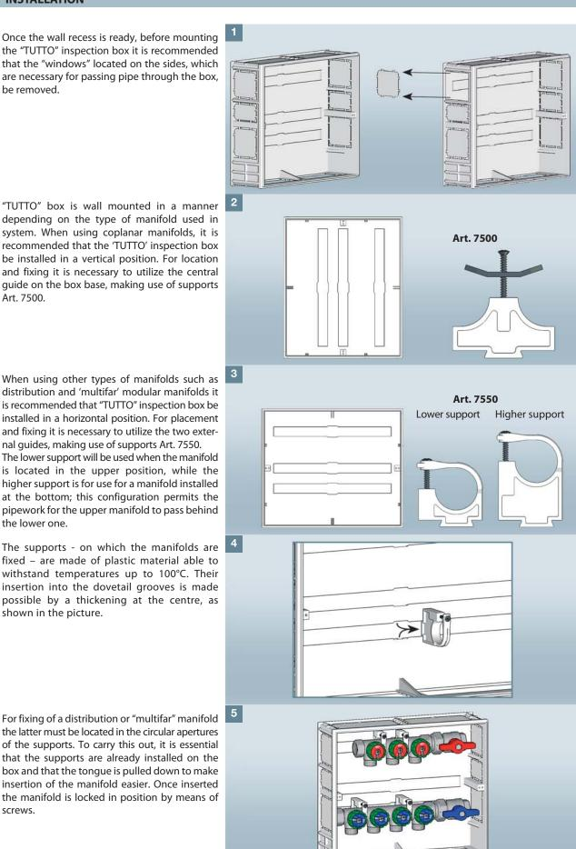
The locking device for coplanar manifold is even simpler. Once the supports are located in the guides, the manifold is laid on them and locked by a screw, which tightens a specially shaped plate in such a way as to centre the manifold on the support.
